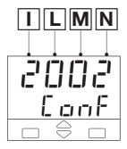
The configuration code can be displayed on the front panel, following the instructions at page 21 section 4.2.2.
