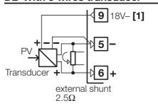
[1] Auxiliary power supply for external transmitter 18Vdc ±20% /30mA max. without short circuit protection
