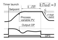
[1] When the Timer is not running the control output is forced to zero, also before the Timer launch
