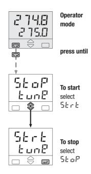
The green led MAN blinking goes on when the Fuzzy Tuning is in progress. At the end of this operation, the calculated PID terms parameter are stored and used by the control algorithm and the controller goes back to the operator mode. The green led MAN becomes off.
